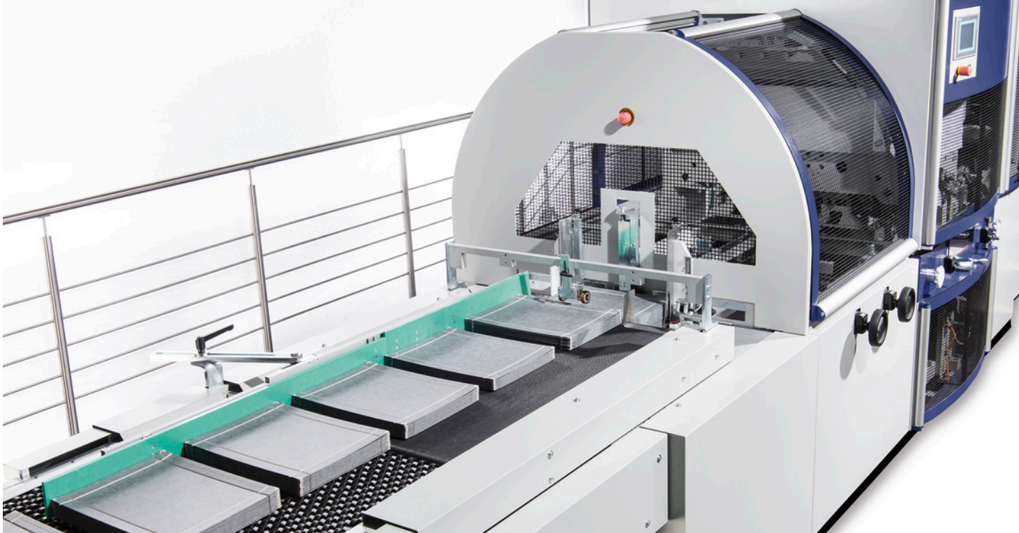
Infeed CF 500 of cross grooved boards in Box Line Puncher
