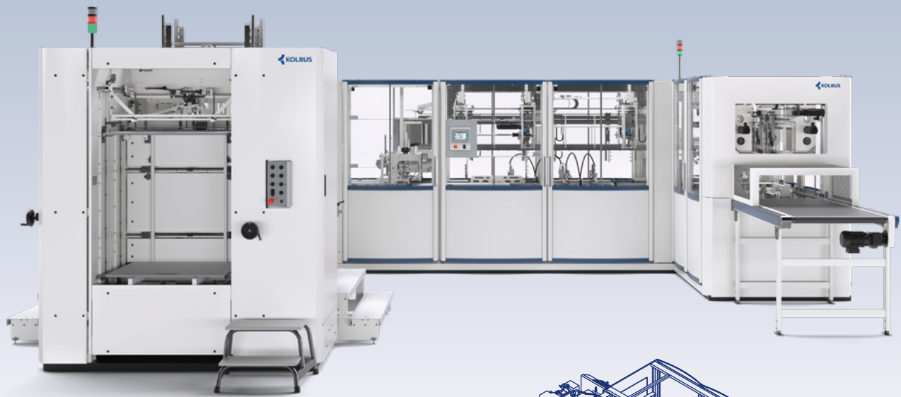
BLT 200 and Box Line Wrapper BLW 200 for forming and laminating boxes
