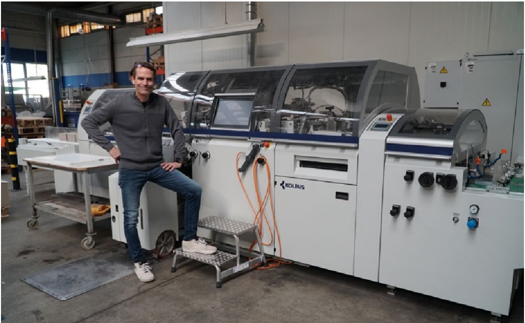
Sascha Terbeck with his new Kolbus DA 370, the fifth of its kind at Terbeck and equipped, among other things, with a cardboard cutting device and a non-stop panel feeder.
